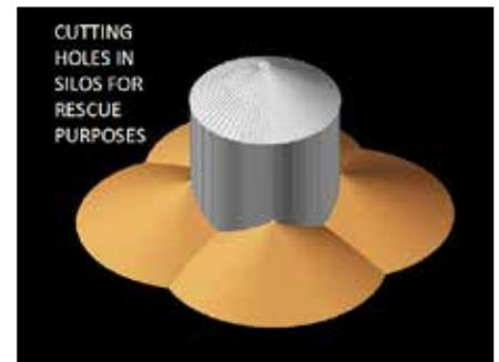
*The most effective and safest means of emptying grain through steel bin walls is to cut four holes around the tank at exactly 90-degree intervals. Illustration courtesy of SCAFCO Grain Systems Co.*
